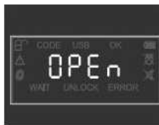
door mechanism will release
